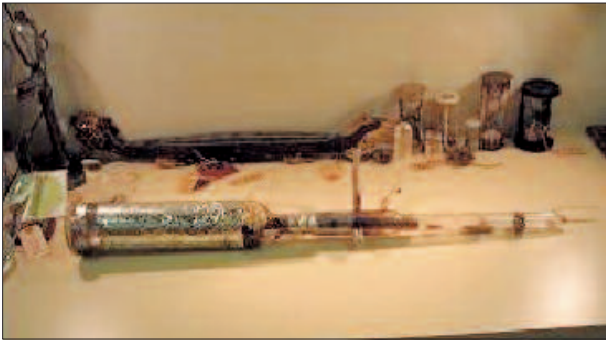
Fig. 4. The cathode ray tube used by Guye and Lavanchy (courtesy of The Geneva Science Museum).
