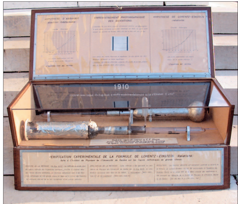
Fig. 7. The wooden cabinet with Guye's two cathode ray tubes (courtesy of The Geneva Science Museum).
